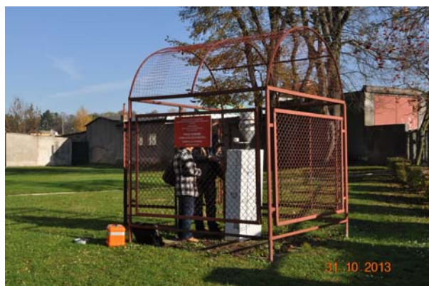
Photography IX.3. Air pollutants measurements with the use of dust sampler and automatic air pollution stations (source: WIOŚ in Szczecin)
