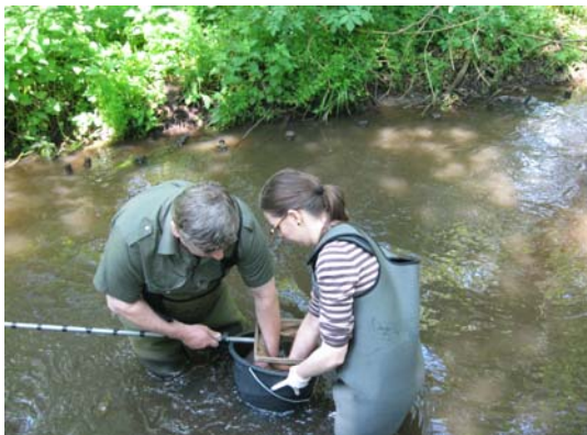
Photography IX.1. Sampling of water from the rivers and groundwater (source: WIOŚ in Szczecin)
